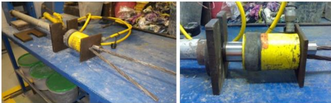
Figure 4.3 – Pull-out test (left); Hidraulics cylinder pulling the cable (right).
